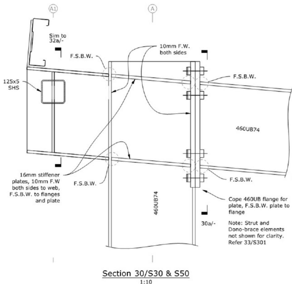
This knee joint was designed to the SONZ Steel Advisor – Moment End Plate – Column Side (CON1001) principles. It is clearly detailed and contains enough information for construction and checking.
