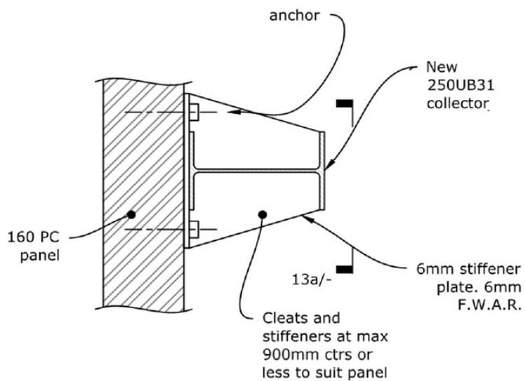
Here, the collector beam has been designed as a part as per MBIE determination 2013/057. The beam also has rotational restraint and can yield.
