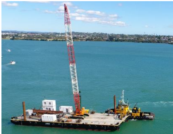
Figure 2: Floating Flat Top Barge (FTB)
