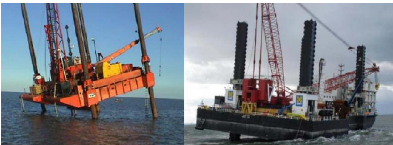
Figure 4: Examples of JUB spud leg punch through
