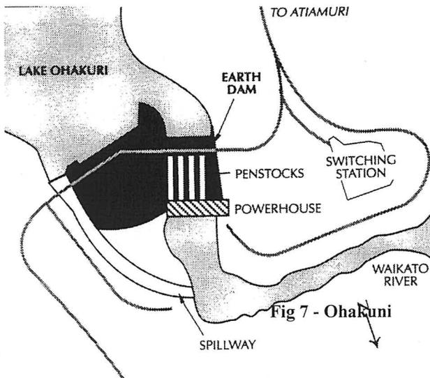
The site appeared to be ideal for an arch dam but the strength of the rock for the right bank abutment was doubtful so a gravity dam was considered. Excavation of the river bed revealed a deep hole that had not been identified in the investigation, so it was decided to build an earth dam with concrete spillway in the right bank and intake structures on the left.
