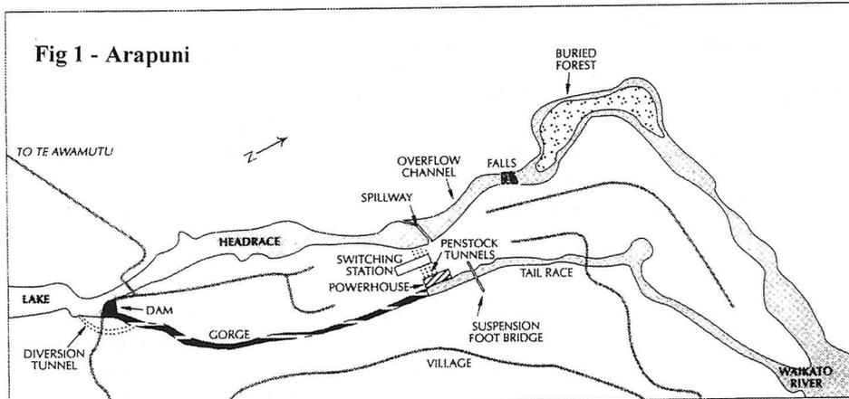
stations on the river to be founded on ignimbrite rock which presented problems of various sorts with all the schemes where it was involved. Geologists maintain that ignimbrite had been erupted in the form of a viscous cloud of particles, which, on being deposited in sheets (or layers) of varying depth, shrinks and cracks on cooling. The configuration of the underlying country varied and determined the nature of the cracking through differential settlement.
