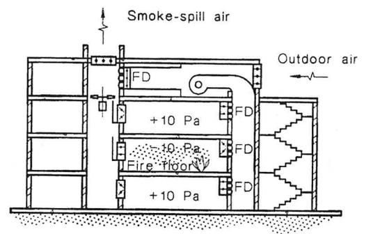
Figure 3: Smokespill fans and arrangement
