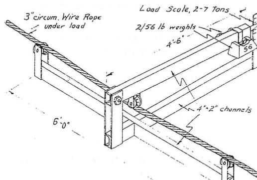
Fig. 3: Isometric view of wire load gauge.
