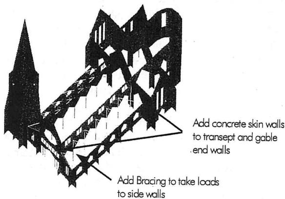
**Fig 7: Christchurch Cathedral – remedial solution: addition of concrete skin walls to Transept and gabled end walls and bracing to take loads to side walls**
