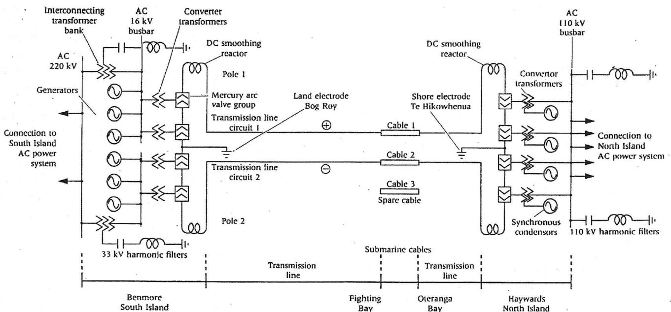
New Zealand HVDC Scheme - Simplified Single Line Diagram
