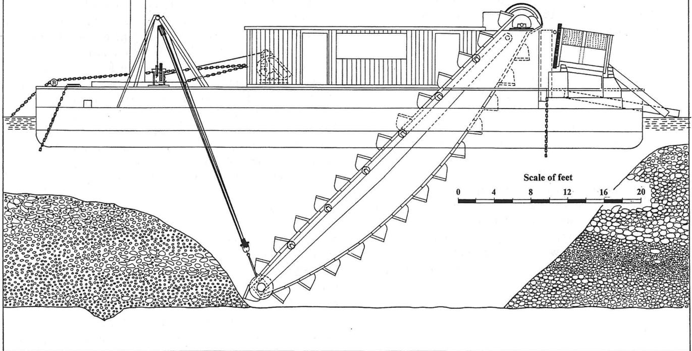
In July 1881, the “Eureka” was launched above Alexandra at a cost of £3,000. However, the boiler and engine were “old worn-out ...much too large” and buckled the pontoon. Coal consumption was also excessive. As a result the “Eureka” was soon converted to a current wheeler (1).
