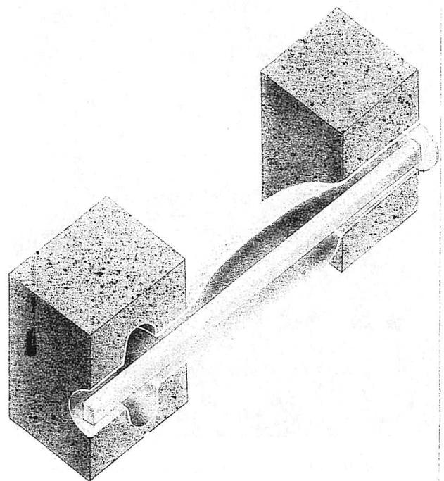
**Fig 9: Basic type of Cintec Anchor, comprising stainless steel anchor and fabric sock which expands inside the cavities of the masonry**
