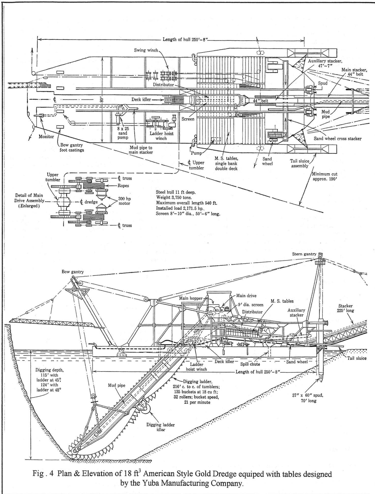
Fig. 4 Plan & Elevation of 18 ft<sup>3</sup> American Style Gold Dredge equipped with tables designed by the Yuba Manufacturing Company.
