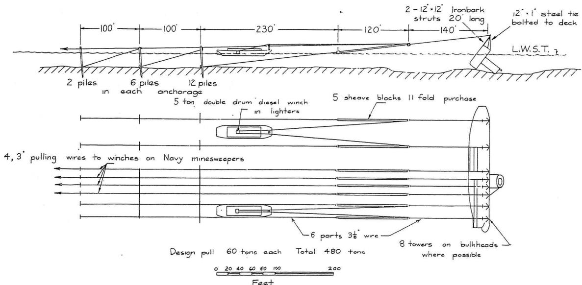
Fig. 2: Layout of equipment for the righting operation.
