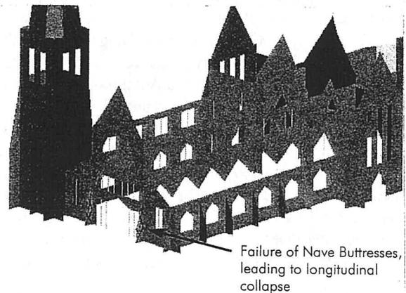
*Fig 6: Christchurch Cathedral – time history non-linear analysis identified weakness in the Nave Buttresses which would lead to longitudinal collapse. Columns in the aisle are flexible and so resist very little earthquake loads. Roof not stiff enough to transfer the Nave wall inertia loads to the exterior walls.*
