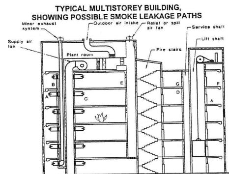
Figure 2: Smoke leakage paths
