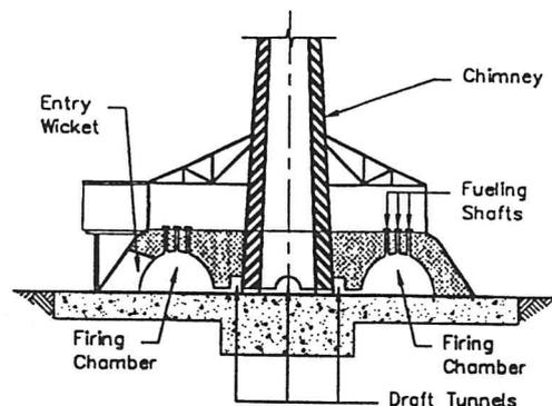
Figure 1 Kiln Cross Section
