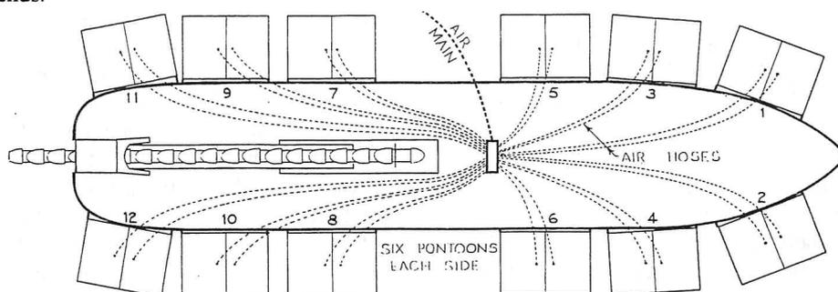
Fig. 6: Arrangement of camels around hull.
