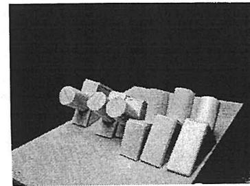
Figure 6 The shoes - concrete wedges shoring props
