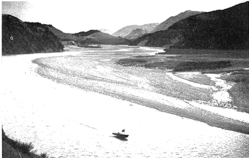
A jet boat at 25 m.p.h. in the Hope River, Canterbury, in water which seldom exceeds 12 in. in depth and often in the shallows of rapids only two or three inches. These are normal operating conditions for the jet boats which draw very little water at speed.
