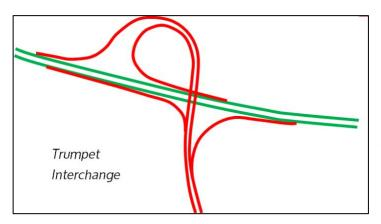
In the same project, when driving down the new expressway, a trumpet interchange was encountered which was built backward. If you drove straight on the trumpet design interchange, you ended up heading in the wrong direction on the expressway. Theoretically and practically, it made no sense.
