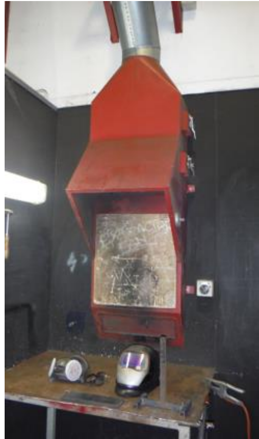
Figure 1: LEV at a metal workers training facility
