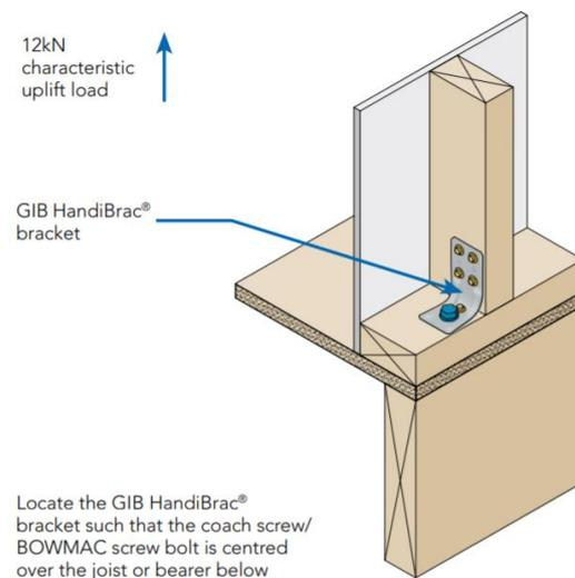
Figure 2: HandiBrac on external joist
