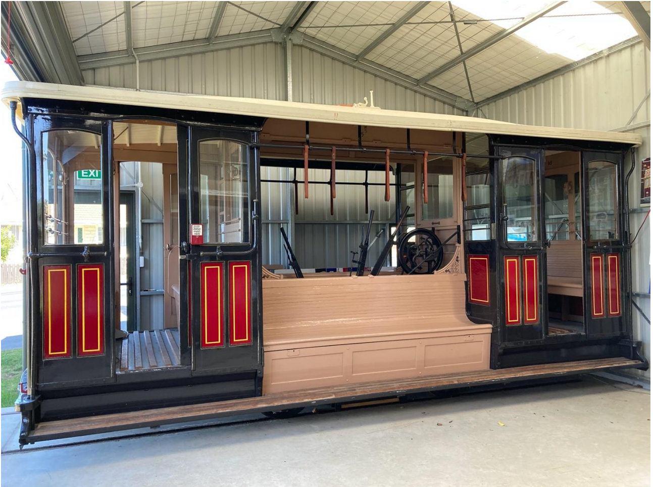
[Figure 6] Restored Roslyn cable car at the Cable Car House, Mornington. Note Fell brake handwheel along with grip lever and regular brake levers. (Photo G M Browne, Sep 2021).
