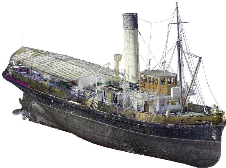
[Figure 4] Final unified point cloud of the Tug Lyttelton as scanned by the Leica RTC360
