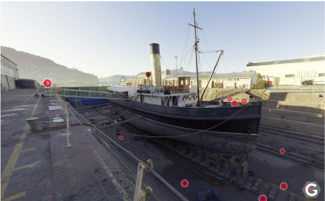
[Figure 5] An example of the 5K HDR panoramic images captured by the RTC360. The red spheres show a sub-selection of the setup locations used to capture the point cloud and panoramic imagery.
