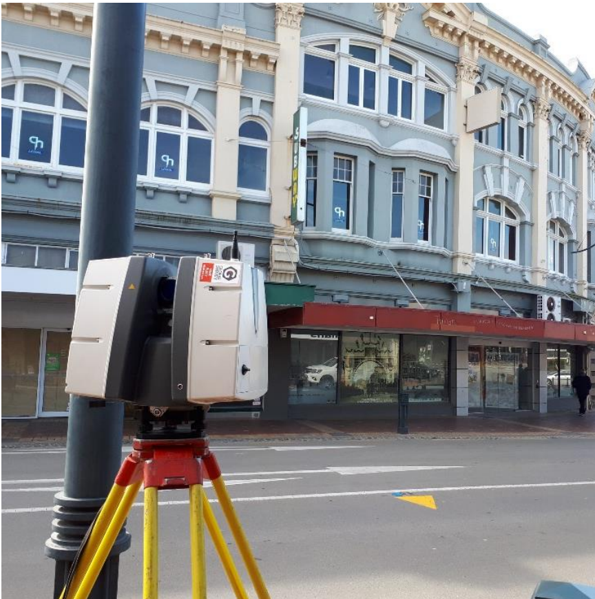
[Figure 2] A survey-grade Leica P40 Laser Scanning capturing a historic building facade
