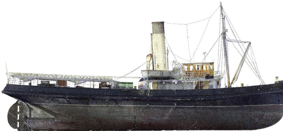
[Figure 6] An orthographic image of the unified point cloud
