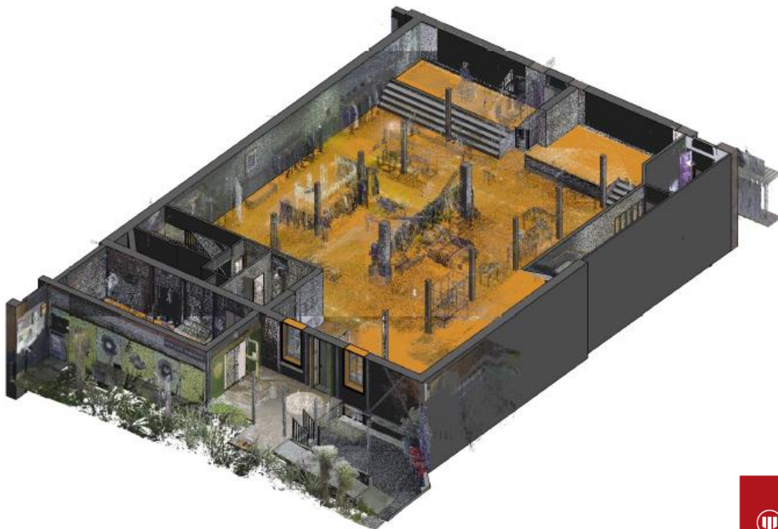
[Figure 12] The 3D model overlaid on the point cloud it was extracted from
