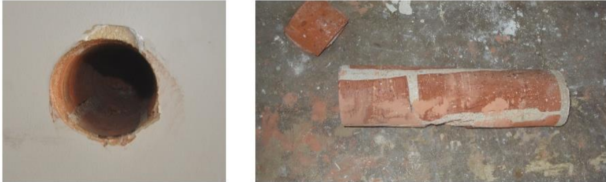
[Figure 7] Photos of existing URM interior wall core samples, illustrating their solid construction with no internal cavity.
