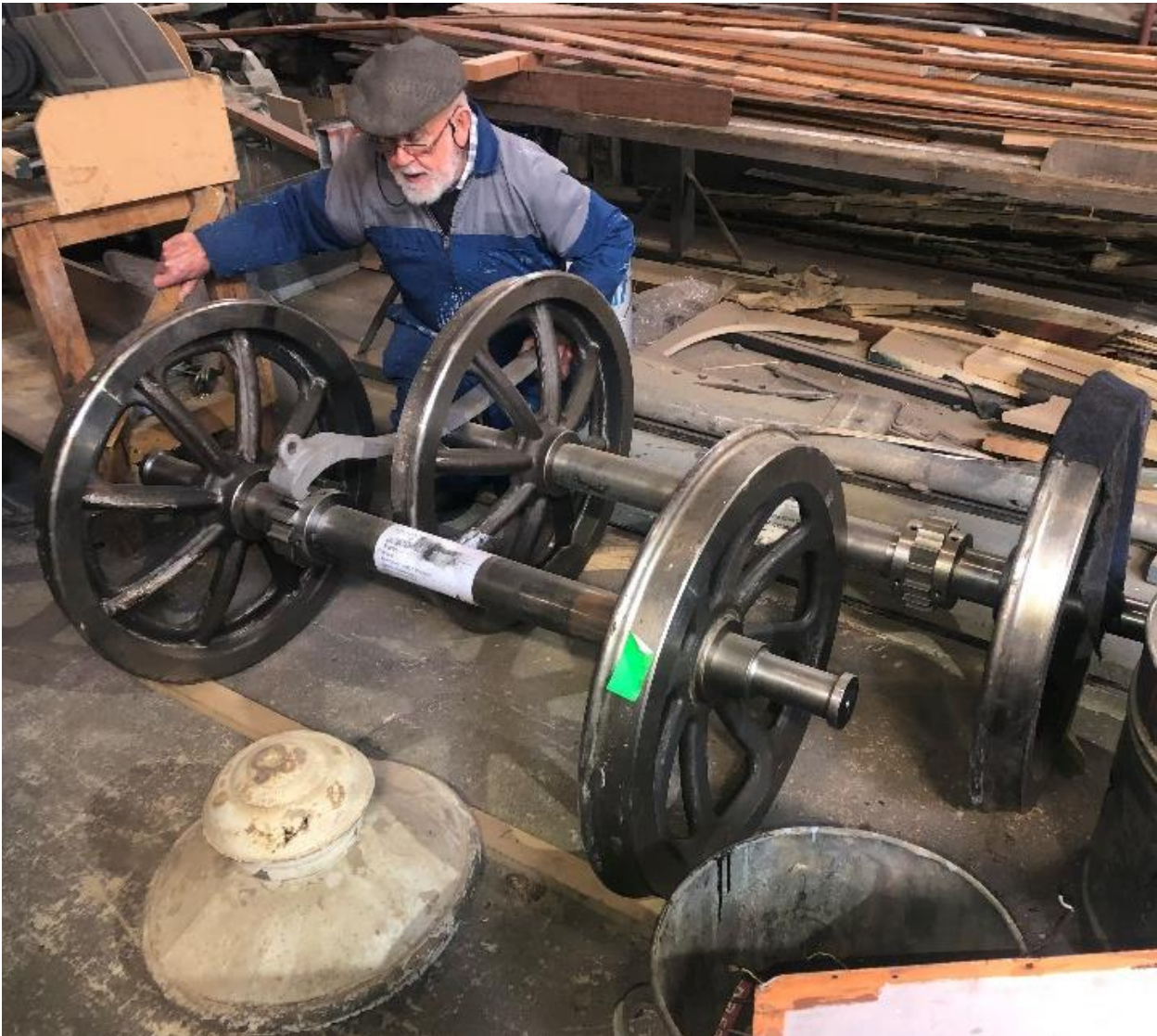
[Figure 23] Don McAra holds a Pawl (gray) into a Ratchet in the 'Tramways Historical Society Tram Barn and Workshop', Ferrymead Christchurch; where Mornington Car 103 is being restored. Photo: ID MacGregor, August 2021.
