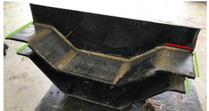
Figure 7 – Photo showing part of the draw beam after failure. This view is looking from the front of the draw beam, ie towards the trailer. Green lines indicate locations of failed welds to the side plates, and the red line indicates another crack.
